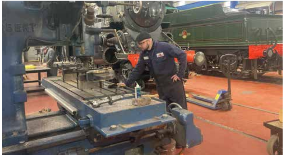
Will Marsh machining the new coupling rod bushes for 75069. Lesley Carr
